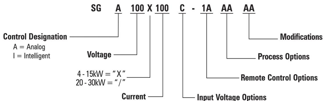
(For units with greater than 3 digits, Voltage/Current is represented in numeric format, e.g., above "100" represents 100A. For units at 1000 and above, the voltage is represented by the format "XKX", e.g. 1K2 = 1200V and 1K0 = 1000V)
