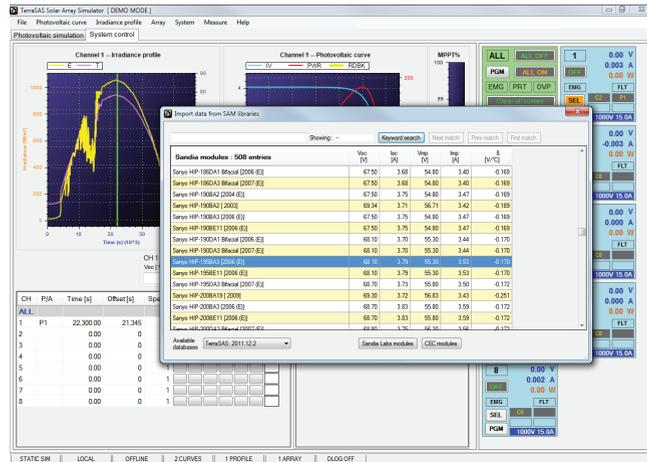
Import module data from embedded Sandia database and create I-V Curve
