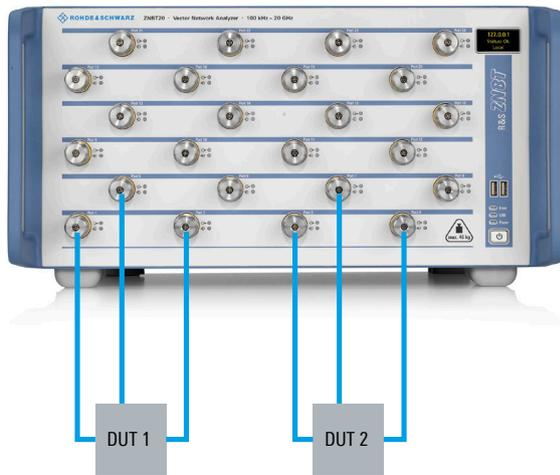
stopband, on the other hand, high output power levels and narrow IF bandwidths are needed to provide the required dynamic range. The instrument's segmented sweep function allows the sweep range to be divided into an almost unlimited number of segments. Sweep parameters such as test point spacing, IF bandwidth and generator power can be defined separately for each segment and accurately matched to the task at hand, optimizing measurement speed and accuracy.
