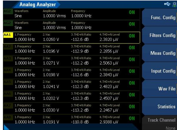
Figure 5. The U8903B's GUI, showing 8 analyzer channel measurements.
