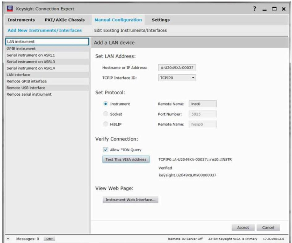
Figure 3. Manual configuration to add the LAN power sensor's LAN connection
