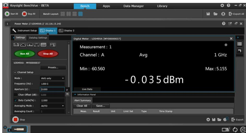
Figure 6. Time-gated average power of pulse width signal (1.2 ms) with aperture time of 10 ms and duty cycle of 12%
