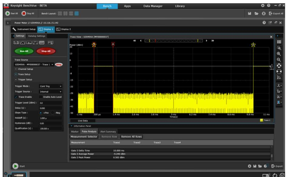
Figure 10. Pulse period measurement (delta time, average and peak) shown in Pulse Analysis table (on top of pulse width measurement)
