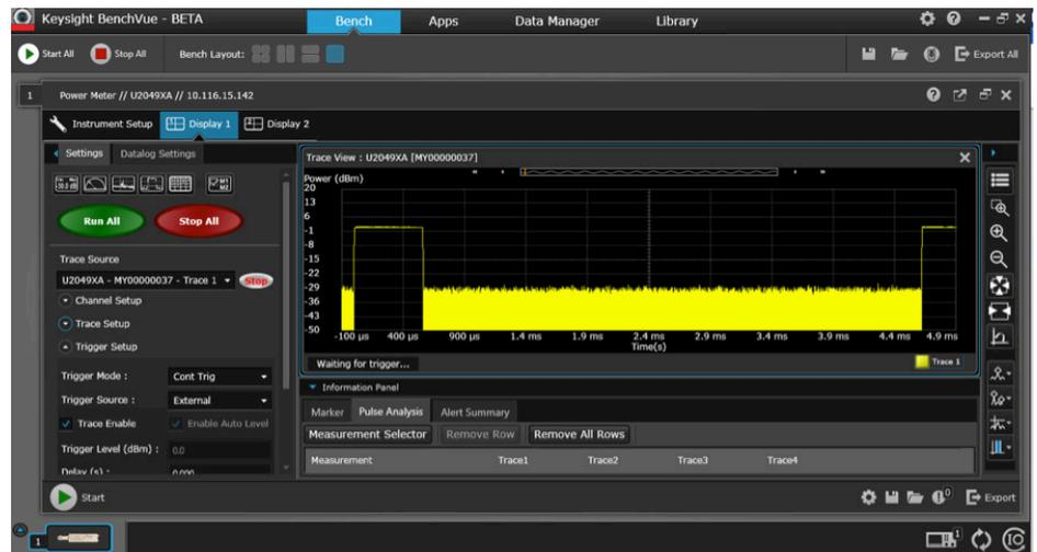
Figure 17. Trace view display capture entire GSM waveform signal
