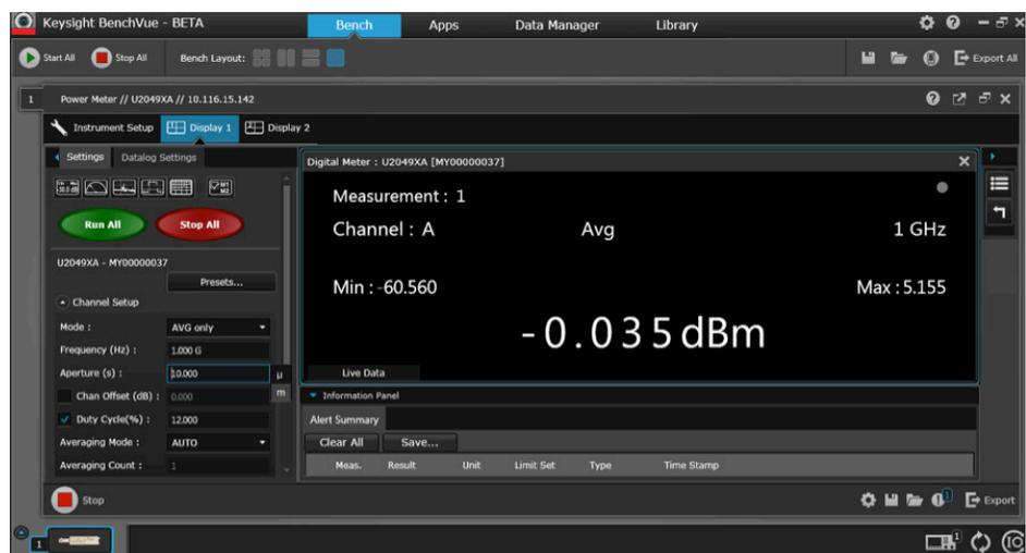
Figure 7. Time-gated average power of pulse width signal (1.2 ms) with aperture time set to 1.2 ms in external triggering mode
