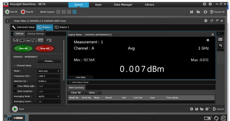
Figure 4. Average power measurement using BenchVue software Power Meter App
