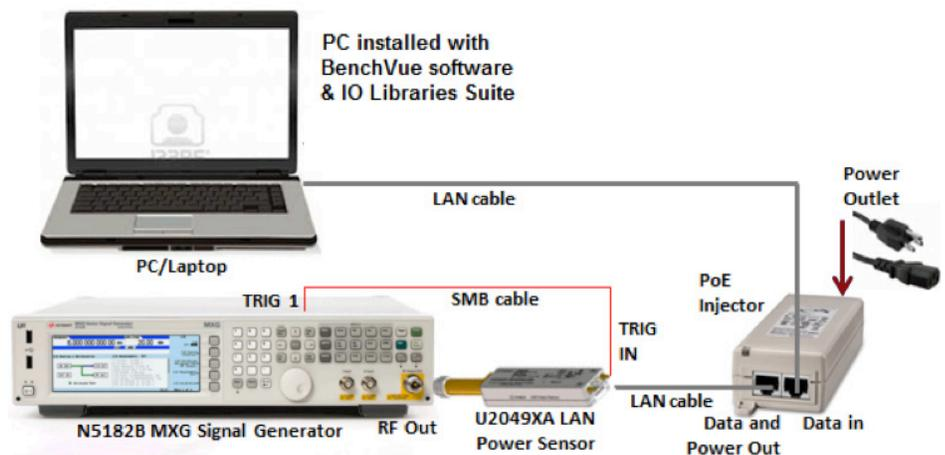
Figure 1. U2049XA LAN power sensor connection diagram with PoE injector
