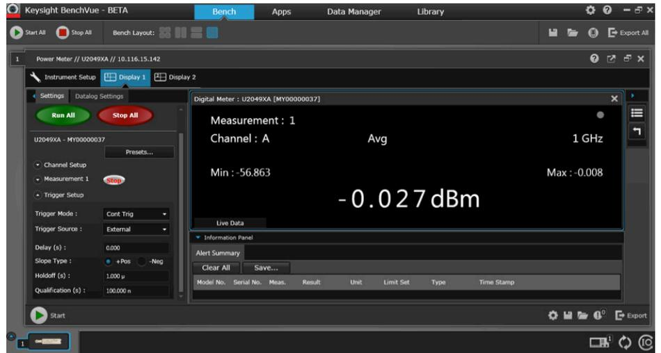
Figure 16. Average power of GSM time-gated signal using aperture time feature in external triggering mode
