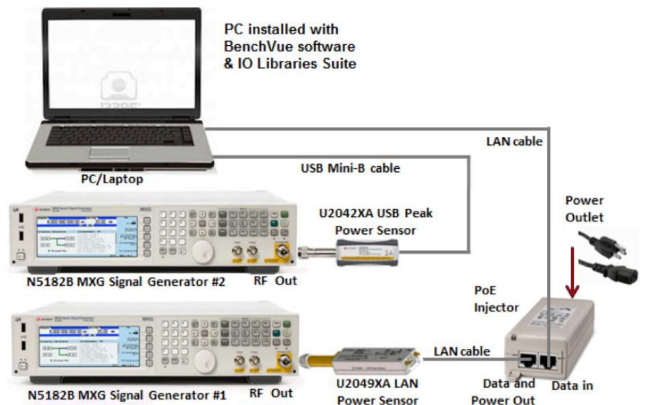
Figure 21. Set up diagram of the U2049XA and U2042XA power sensors with two signal generators
