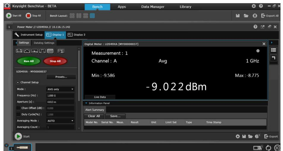
Figure 15. Average power measurement with aperture time set to 4.613 ms to capture entire GSM waveform signal
