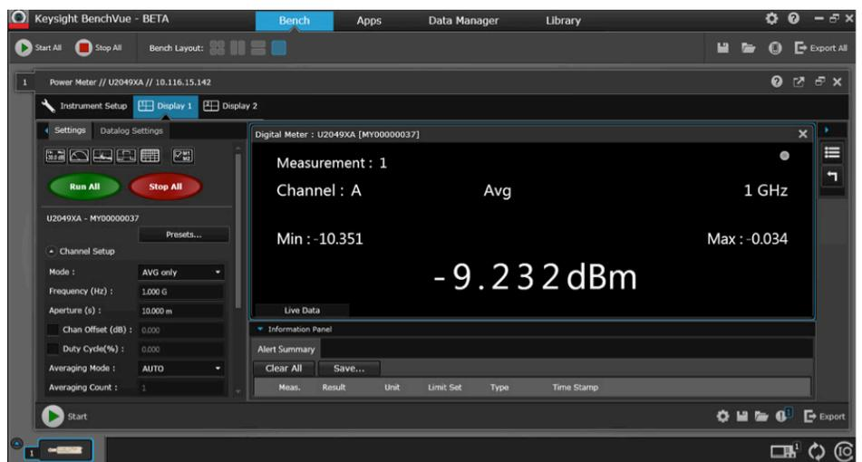
Figure 5. Average power measurement with aperture time set to 10 ms to capture entire pulse signal
