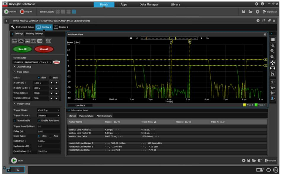
Figure 24. Horizontal line marker indicates the power differential, ~ -7.77 dB between two pulses
