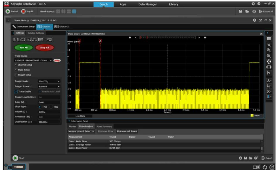
Figure 18. Time-gated measurement on GSM timeslot 0 with Gate 1 feature
