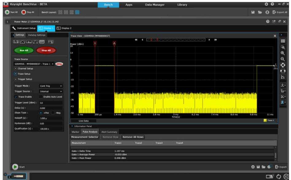
Figure 9. Pulse width measurement (delta time, average and peak) shown in Pulse Analysis table
