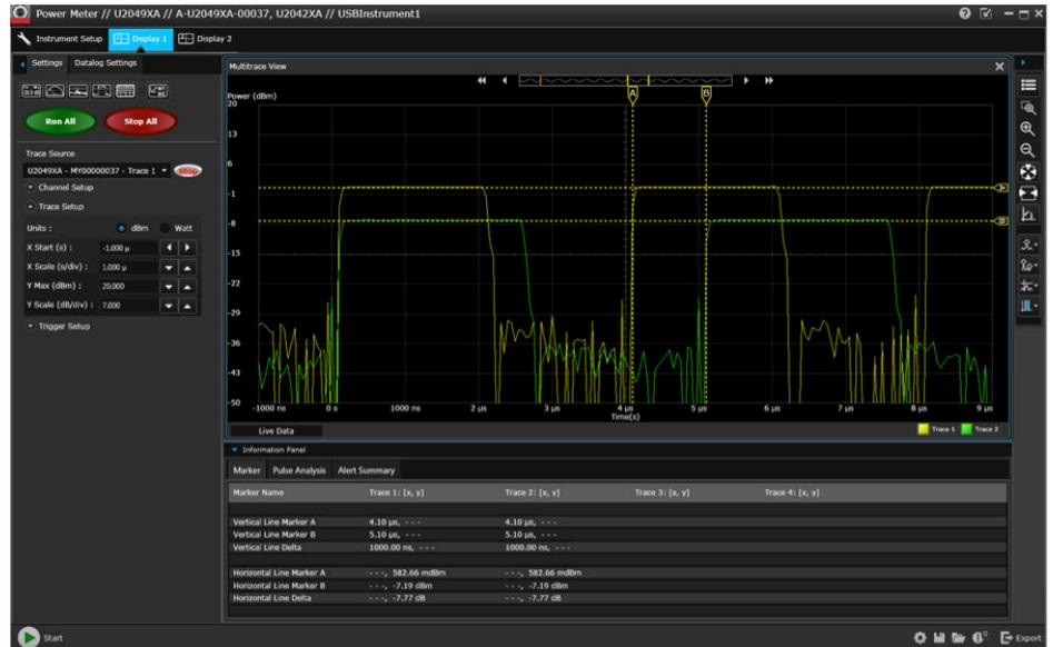
Figure 25. Power Meter App application shown in separate window, which allows the trace graph space to be maximized for better pulse analysis measurement
