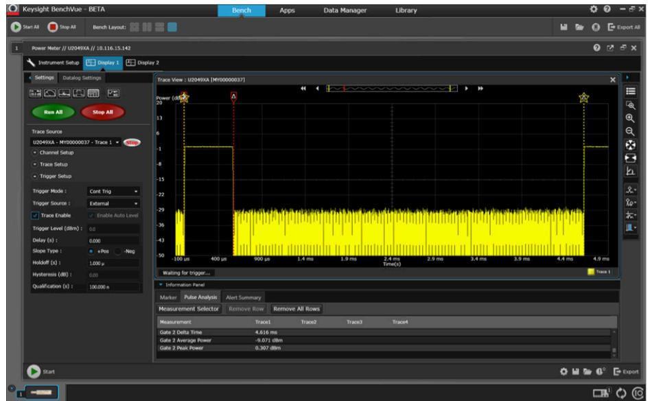
Figure 19. GSM waveform signal 4.613 ms duration show average, peak, and peak-to-average with Gate 2 feature
