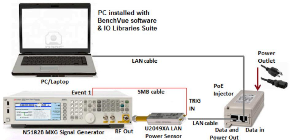
Figure 14. Setup diagram of external trigger port from signal generator to trigger LAN power sensor through its trigger input port
