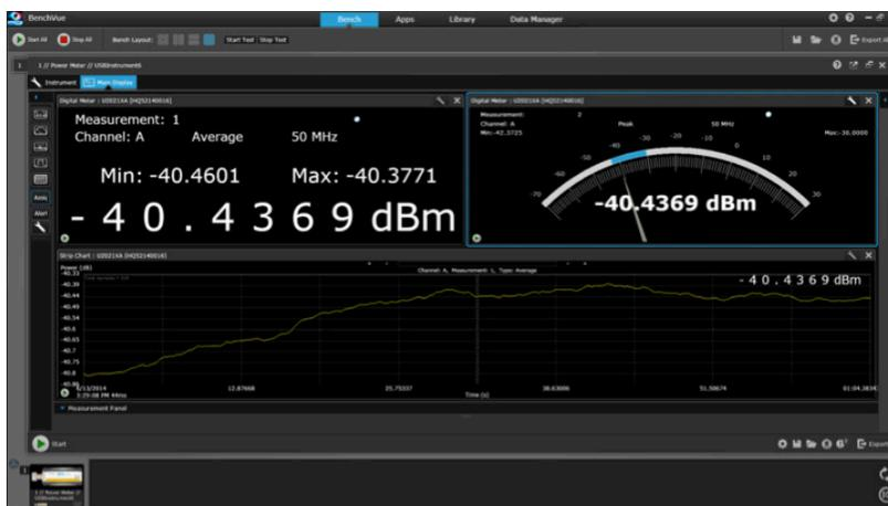
BenchVue software Power Meter App's graphical user interface supports multiple measurement display formats
