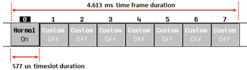
Figure 13. GSM timeslot pattern with timeslot 0 On
