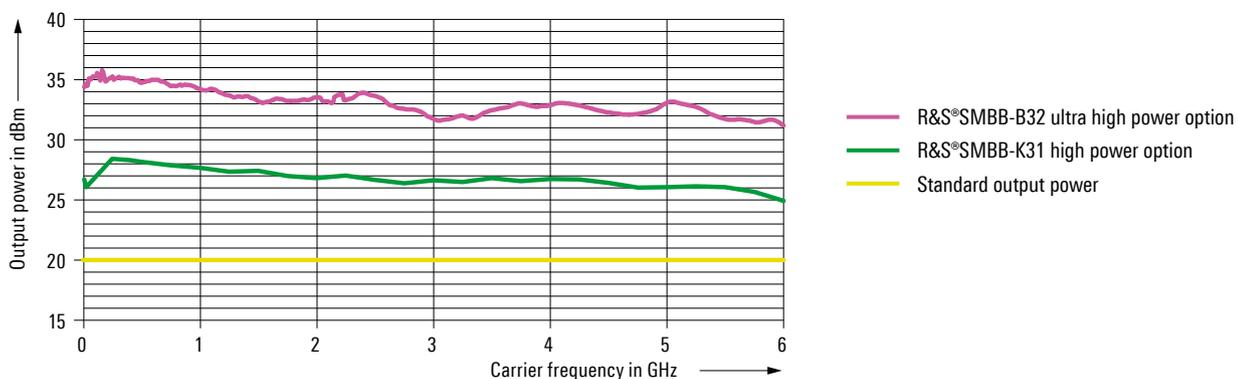
Measured output power for the base unit, with the high power option (R&S®SMBB-K31) and with the additional ultra high power option (R&S®SMBB-B32).
