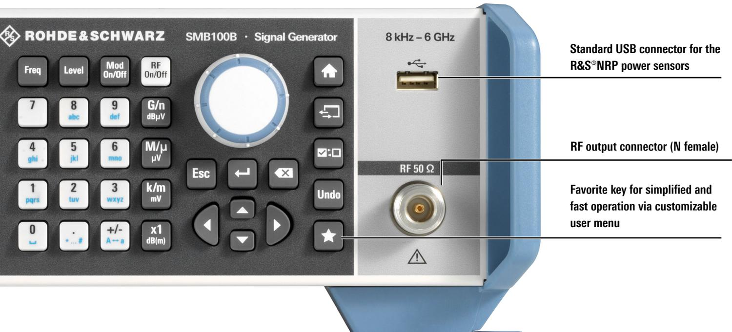
Standard USB connector for the R&S®NRP power sensors
