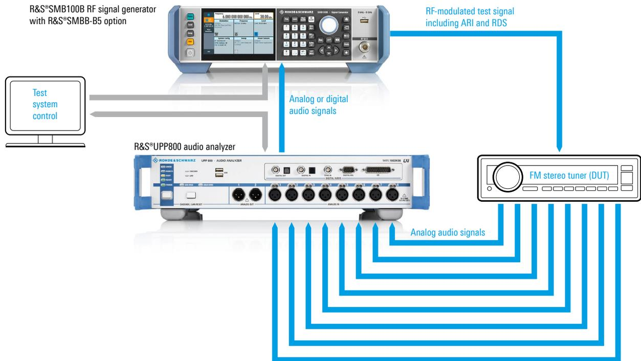
The R&S®UPP800 audio analyzer generates all required audio test signals and transfers them to the R&S®SMB100B, which adds the ARI and RDS test signals and modulates the entire test signal onto the RF carrier. The DUT demodulates the received test signal and outputs the audio signals on all amplifier channels. Measuring these signals with the R&S®UPP800 closes the loop and makes it possible to analyze the overall sound quality of the car radio under test.
