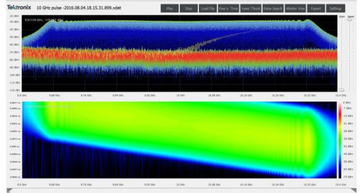
Above is a color-graded spectrum display combined with a 99% overlap spectrogram display as shown on DataVu-PC. You have full overlap/skip control to vary rate and detail of the streaming file for complete visualization of the data.
