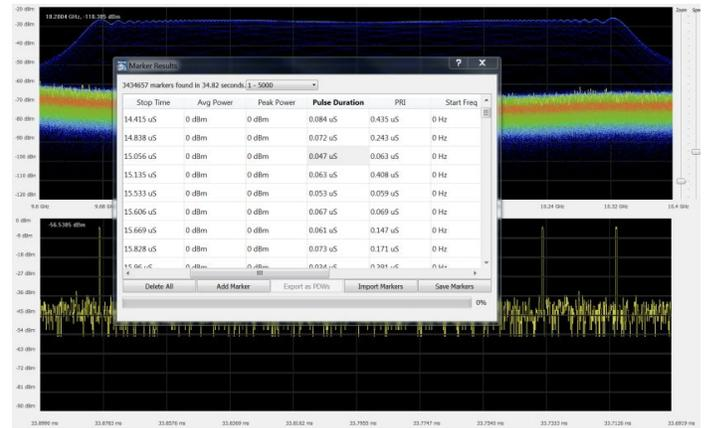
DataVu-PC pulse option provides fast marking of pulses and measurements on large data sets. Above, the results of a pulse search are presented with the pulse measurements of start/stop time, average/peak power, pulse duration, Pulse Repetition Interval (PRI) and start/stop frequencies on up to 2,000,000 pulses. Pulse results can be exported in PDW format for use by other tools.
