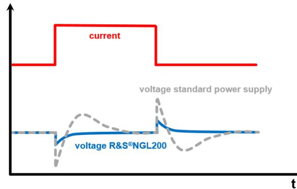
During challenging load conditions, most power supplies react with slow recovery times and overshoots. Specially developed circuits in the R&S®NGL200 series achieve a load recovery time of < 30 µs with minimal overshoot, making them perfect for supplying sensitive components
