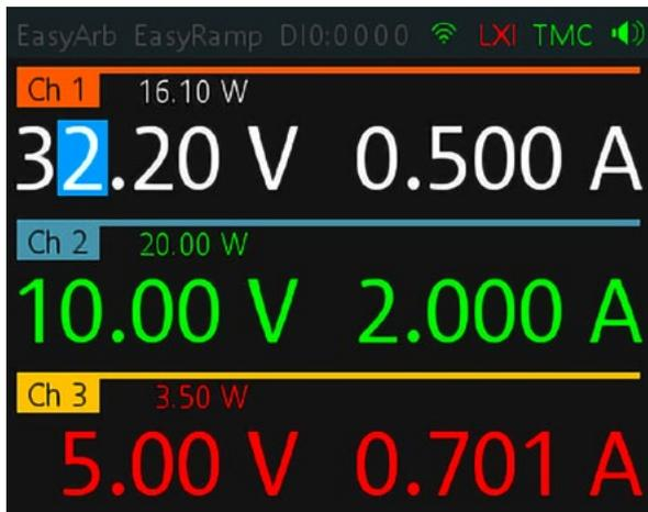
The different operating conditions are marked by colors: constant voltage operation is indicated in green, constant current operation in red, inactive channels are shown in white, a number marked by a blue background indicates that the channel is in setting mode
