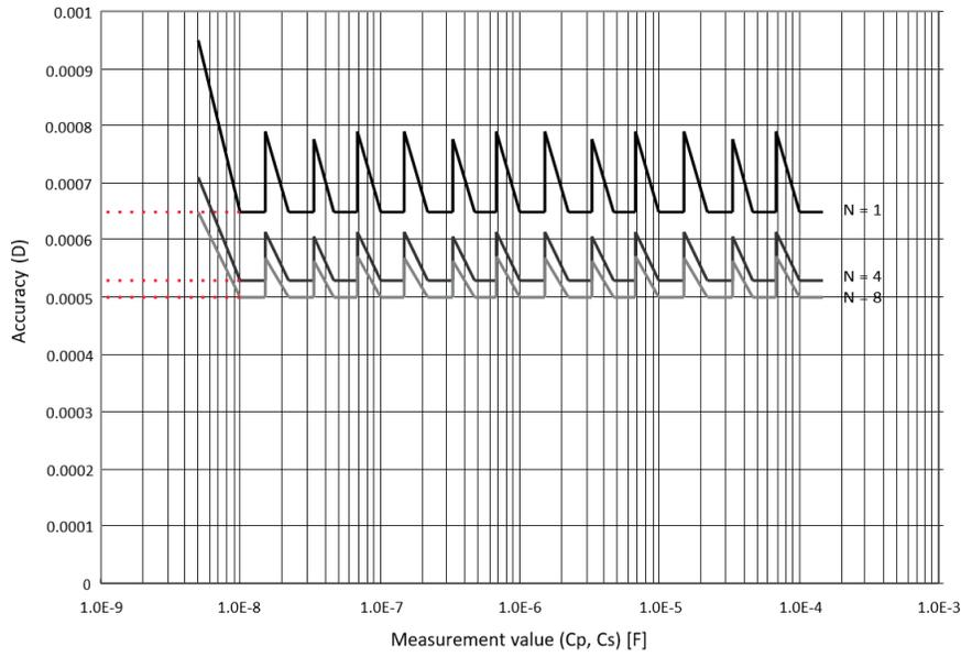
Figure 1. Accuracy of D when measurement frequency is 120 Hz
