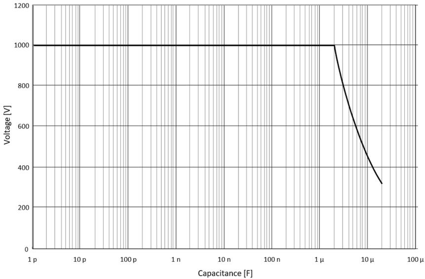
Figure 14. Maximum discharge withstands voltage (typical)
