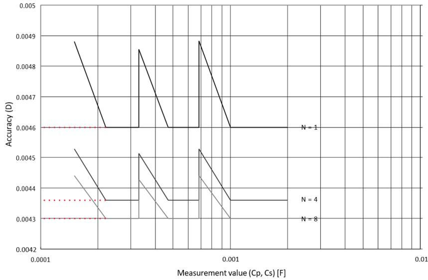
Figure 3. Accuracy of D when measurement frequency is 120 Hz
