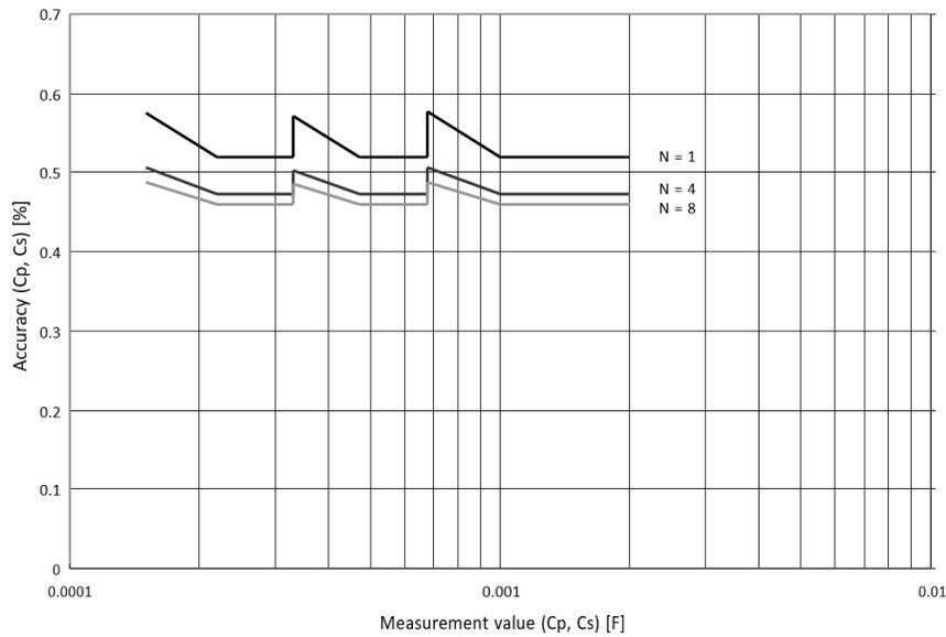
Figure 4. Accuracy of Cp and Cs when measurement frequency is 120 Hz
