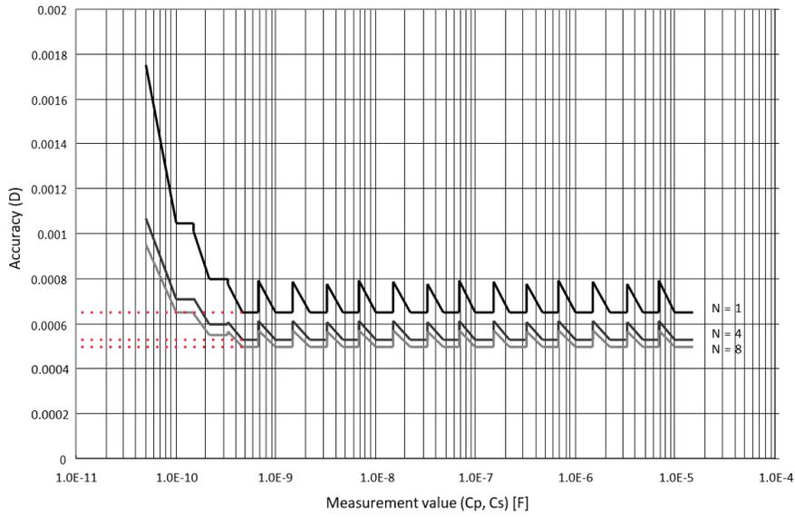
Figure 5. Accuracy of D when measurement frequency is 1 kHz
