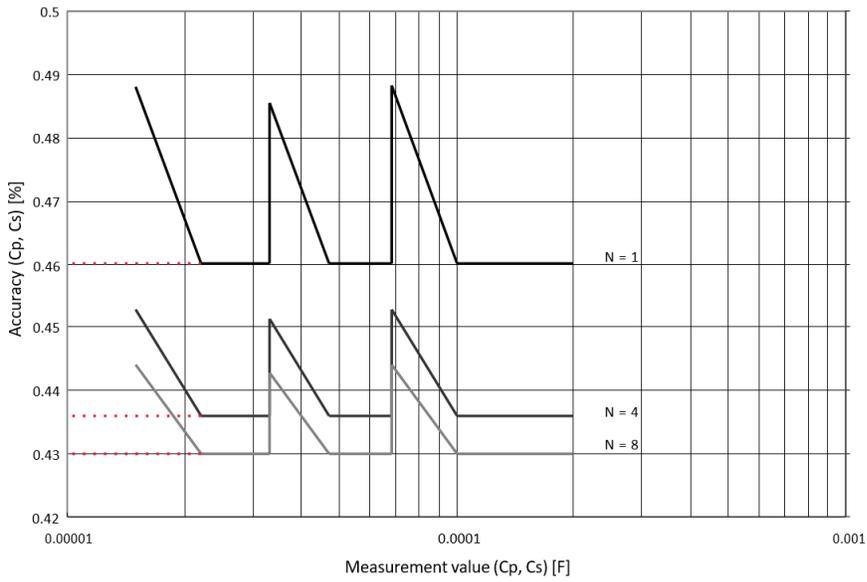
Figure 8. Accuracy of Cp and Cs when measurement frequency is 1 kHz
