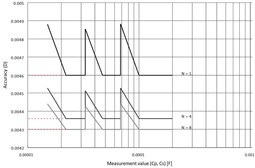
Figure 7. Accuracy of D when measurement frequency is 1 kHz
