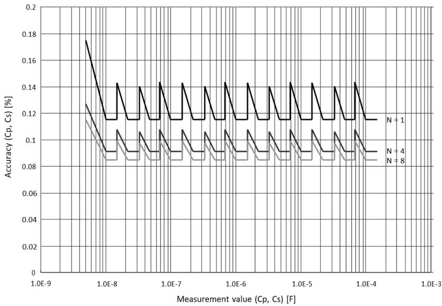
Figure 2. Accuracy of Cp and Cs when measurement frequency is 120 Hz
