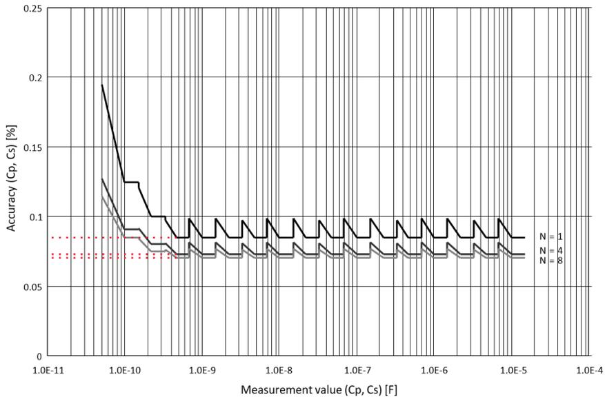
Figure 6. Accuracy of Cp and Cs when measurement frequency is 1 kHz
