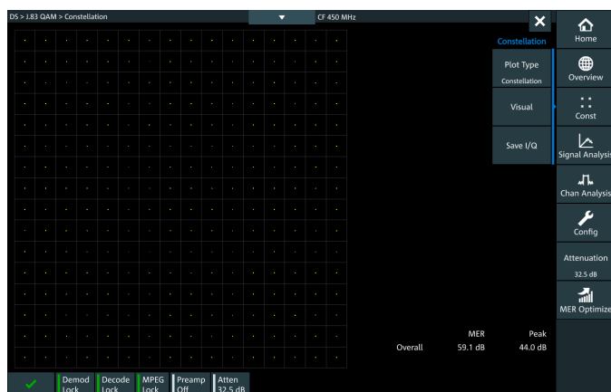
J.83 constellation diagram with 256QAM
