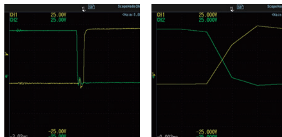
Gate signal waveforms of inverter (20 kHz)
